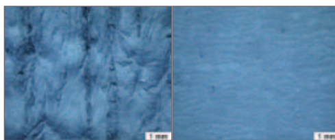
Gussoberflächen: [li] Standardkokillendesign; [re] innovative Hot-Top-Kokille
